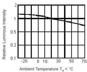
Luminous Intensity vs. Ambient Temperature
