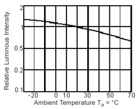
Luminous Intensity vs. Ambient Temperature
