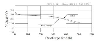
Storage at  $60\,\bot\,$  for 30 days equivalent to storage at room temperature for 18 months
