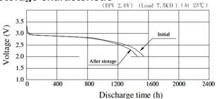
Storage at 60°C for 30 days equivalent to storage at room temperature for 18 months
