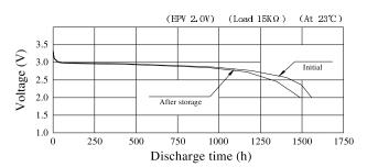
Storage at  $60\,\bot\,$  for 30 days equivalent to storage at room temperature for 18 months
