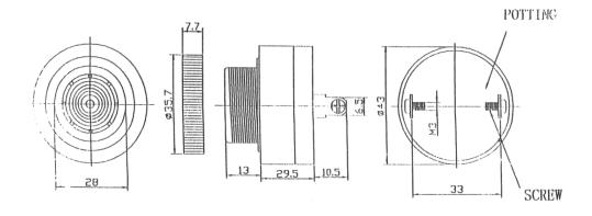
Dimensions : Millimetres Tolerance: ±0.5m
