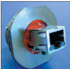
In some applications, a **transversal sealing** for the receptacle is a « must ». This will prevent fluids and dust from going through the receptacle when plug or cap are not mated to the receptacle. The sealed solution (version "S") has a compound at the rear of the receptacle as shown on the picture. For more information, please consult datasheet RJF-RJFTV Environmentally Sealed Receptacles, page 23.
