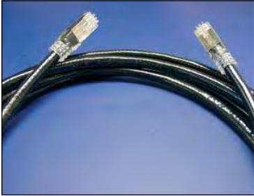
General Construction: A 4 pair, 24 AWG, 100 Ohm SFTP round patch cable, designed to the ISO / IEC 11801 Category 5e requirements (cat 5e on 76m). The cable contains 4 twisted pairs, cabled, double shielded with kevlar reinforcement strands, jacketed in black UV resistant Polyurethane HFFR. Designed for fixed or portable applications in harsh environments.
