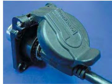
This Self Closing Cap automatically protects the RJ Field square flange receptacles (MIL-C-26482 type), protecting your system from dust and water projections. The same cap can be used to protect USB and IEEE1394 receptacles. A spring automatically closes the upper part of the cap when either the RJ Field plug, RJ45 cordset, USB or IEEE1394 cordset, or USB key are removed from the receptacle.
