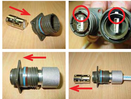
To remove the USB module, insert the removal tool USBF ODE from the front, and push back the module.
