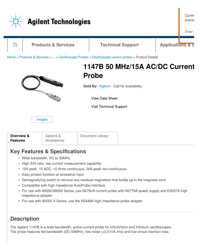
The 1147B is ideal for capturing transient current signals such as those found in motor controllers, switching power supplies, inverters and current amplifiers driving inductive loads.
