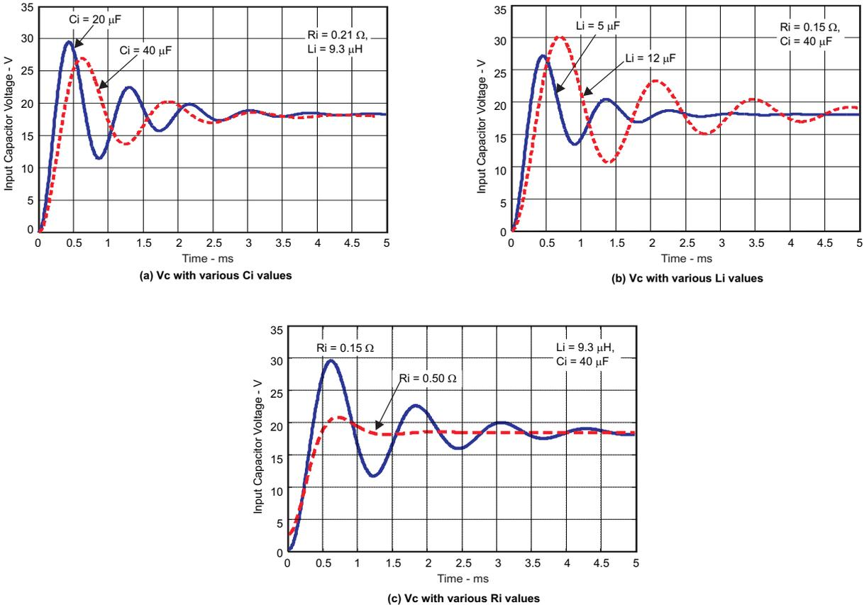
**Figure 30. Parametric Study Of The Input Voltage**
