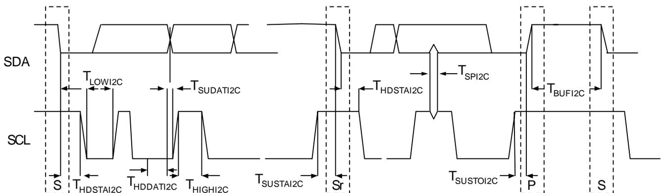
**Figure 3-11. Definition for Timing for Fast/Standard Mode on the I<sup>2</sup>C Bus**
