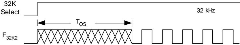
Figure 3-5. External Crystal Oscillator Startup Timing Diagram
