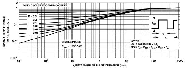
Figure 13. Junction-to-Ambient Transient Thermal Response Curve
