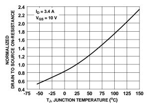
Figure 3. Normalized On-Resistance vs Junction Temperature
