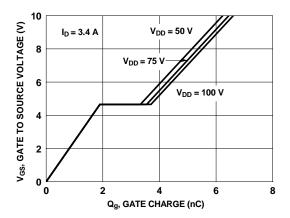
Figure 7. Gate Charge Characteristics
