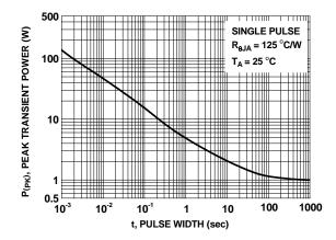
Figure 12. Single Pulse Maximum Power Dissipation
