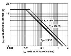
Figure 9. Unclamped Inductive Switching Capability
