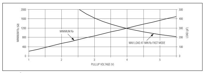
Figure 11. I<sup>2</sup>C Fast Mode Pullup Resistor Selection Chart
