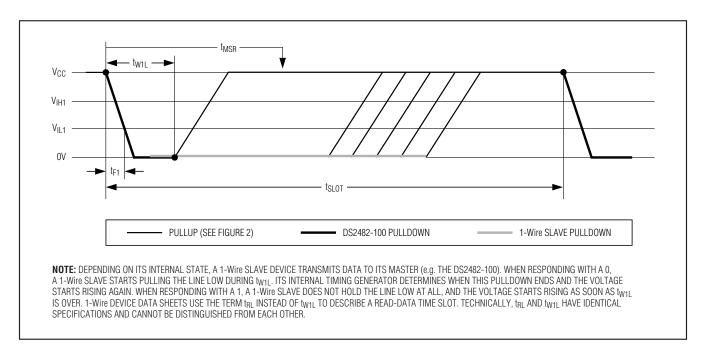
Figure 6. Write-One and Read-Data Time Slot
