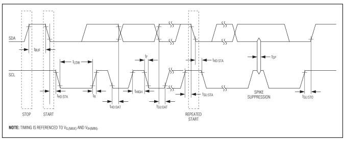
Figure 9. I<sup>2</sup>C Timing Diagram
