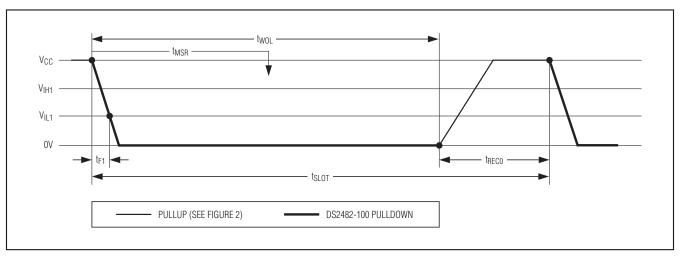
Figure 5. Write-Zero Time Slot
