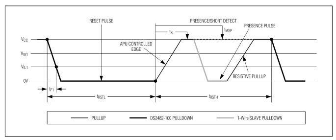
Figure 4. 1-Wire Reset/Presence-Detect Cycle
