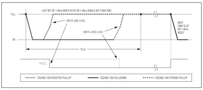
Figure 3. Low-Impedance Pullup Timing
