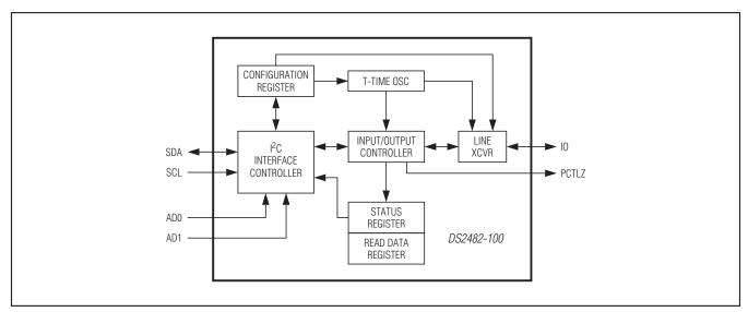
Figure 1. Block Diagram
