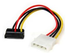
The SATAPOWADPL Molex to 90-degree SATA power adapter features one 4-Pin Molex (LP4) male connector and a left angle, 90-degree SATA power connector (female), which enables you to power a Serial ATA hard drive from a conventional LP4 connection and eliminates the need to upgrade the computer power supply for compatibility with the SATA hard drive.
