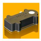
The **UVMICROLOG** is designed for logging of ultraviolet radiation, temperature, pressure and acceleration. Sophisticated microcontroller technology and low noise SiC TOCON based UV detectors allow up to 3 months of permanent measurement and logging without battery charging. The unit can be mounted with a belt or screws.
