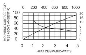
THERMAL RESISTANCE FROM MTG SURFACE TO AMBIENT-C/WATT
