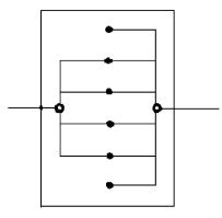
Terminals 1 and 6 are frequently unused, 2 pair (4 wire) cable is normally used in these installations.
