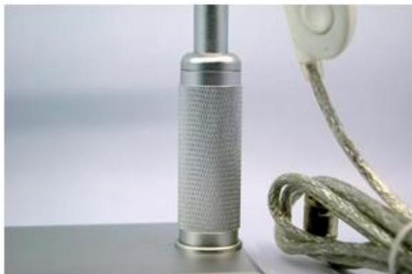
And the pen microscope can be moved up and down by turning the pillar (see left photo) for getting larger or smaller photo area.
