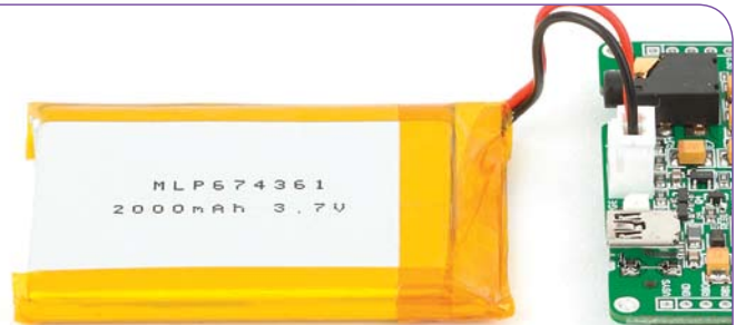
Figure 1-2: Connecting Li-Polymer battery
