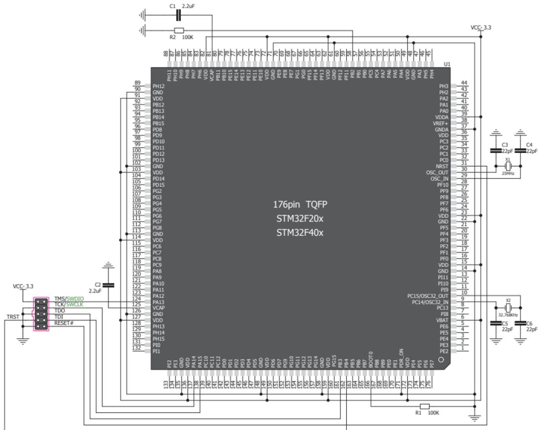
Figure 7-5: Connection schematics for 176-pin STM32F20x/STM32F40x MCU via 2x5 male header
