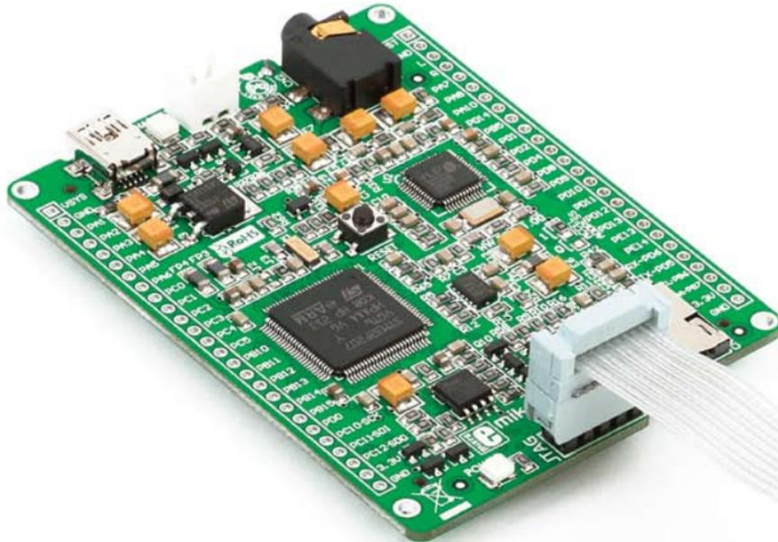
Following examples demonstrate connections with some of the most popular supported microcontrollers. Each one is carefully selected as a representative of the entire family. All MCUs use TMS, TCK, TDO, TDI, TRST, #RESET lines for JTAG programming or SWDIO, SWCLK for SWD (Serial Wire Debug) programming. These lines are located on same microcontroller pins within a family.
