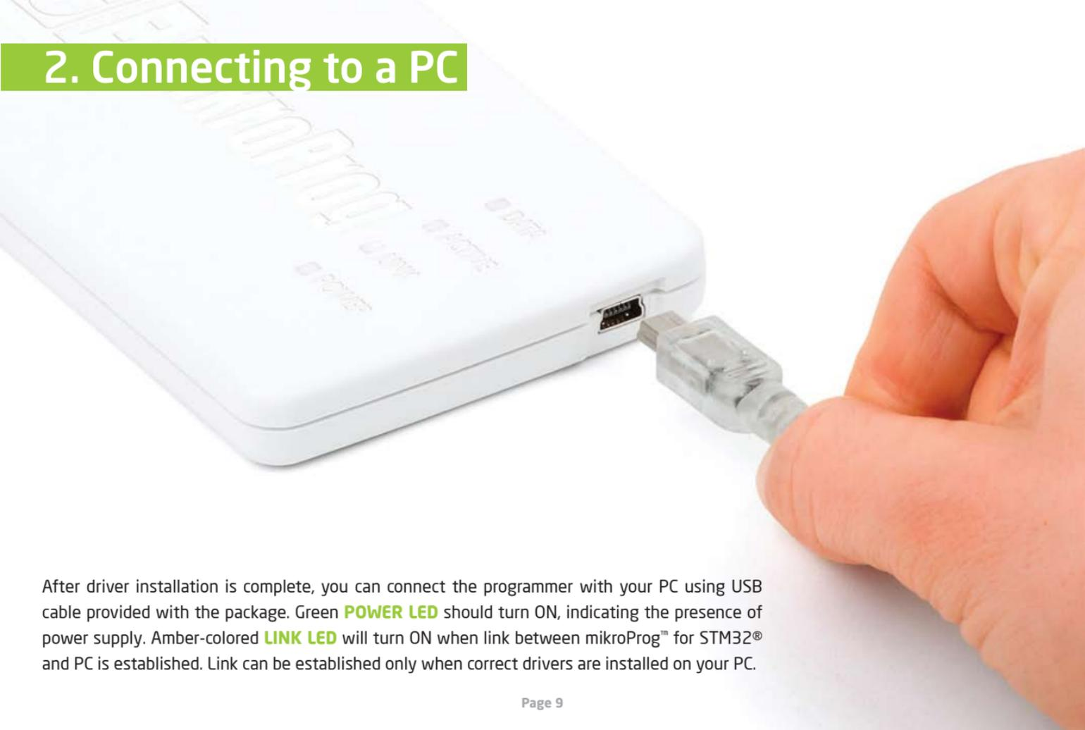
After driver installation is complete, you can connect the programmer with your PC using USB cable provided with the package. Green **POWER LED** should turn ON, indicating the presence of power supply. Amber-colored **LINK LED** will turn ON when link between mikroProg™ for STM32® and PC is established. Link can be established only when correct drivers are installed on your PC.
