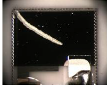
Active sensor area with a scratch
