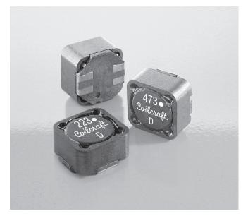
The MSC1278 coupled inductors are designed with high leakage inductance for use in SEPIC applications. The loosely coupled windings (K  $\approx$  0.8) improve SEPIC efficiency by reducing circulating current and provide twice the ripple current reduction of separate inductors.
