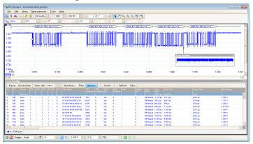
The PicoScope 3000 Series, with its deep memory, is ideal for serial decoding as it can capture thousands of frames of uninterrupted data.
