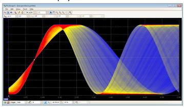
See old and new data superimposed, with new data in a brighter color or shade. This makes it easy to see glitches and dropouts and to estimate their relative frequency. Choose between analog persistence and digital color, or create a custom display mode.
