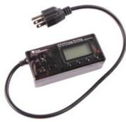
This smart plug reference design features the MSP430AFE253 and monitors electricity consumption for any household electrical appliance. Incoming AC voltage, current, frequency, active power, reactive power, apparent power, power factor and energy consumption in kWh is measured and displayed on the LCD.
