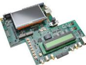
Full-featured application development kit for evaluating the functionality of TI's highly integrated, energy-efficient Sitara™ ARM® AM1808, AM1806 and AM1802 application processors. Also features Bluetooth® and Wi-Fi connectivity with integrated LCD, touch and backlight display.
