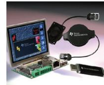
This intelligent-display, single-board computer is a reference design for a complete 3.5" QVGA touch-screen user interface for control, automation and instrumentation applications. It is based on the feature-rich Stellaris® LM3S9B92 microcontroller featuring Ethernet, USB OTG/host/device and CAN.
