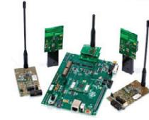
The CC-6LOWPAN-DK-868 is a complete development kit for a sub-1-GHz 6LoWPAN system. It supports the 868-MHz frequency band and can quickly be reconfigured in software for operation in the 915-MHz ISM band. Additional evaluation module kits can be purchased separately to support other frequencies.
