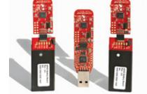
This kit provides the perfect introduction to 2.4-GHz ZigBee wireless sensor networks. Designed for engineers who want to get familiar with this technology without having to port a lot of software to get up and running.
