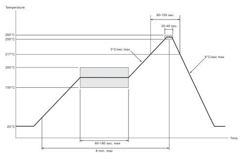
Figure 3-1: Maximum Pb-free Solder Reflow Profile (Preferred)
