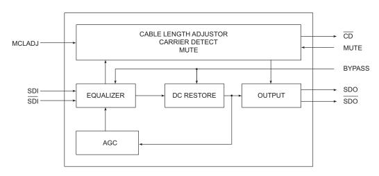
Figure A: GS1574A Functional Block Diagram
