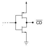
Figure 5-5:  $\overline{\text{CD}}$  Circuit
