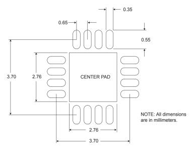
The Center Pad should be connected to the most negative power supply plane for analog circuitry in the device (VEE\_A) by a minimum of 5 vias.
