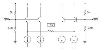
Figure 5-1: Input Equivalent Circuit
