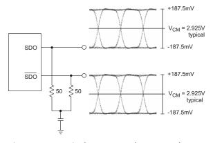
Figure 6-1: Typical Output Voltage Levels
