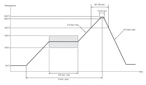
Figure 3-2: Standard Pb Solder Reflow Profile
