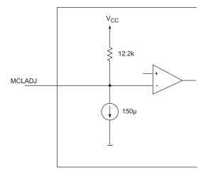
Figure 5-2: MCLADJ Equivalent Circuit
