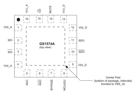
Figure 1-1: 16-Pin QFN
