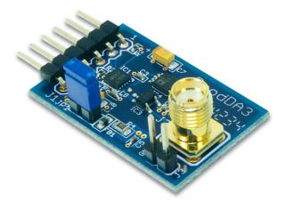
allow the PmodDA3 to plug directly into the system board or to connect via a Digilent sixwire cable
