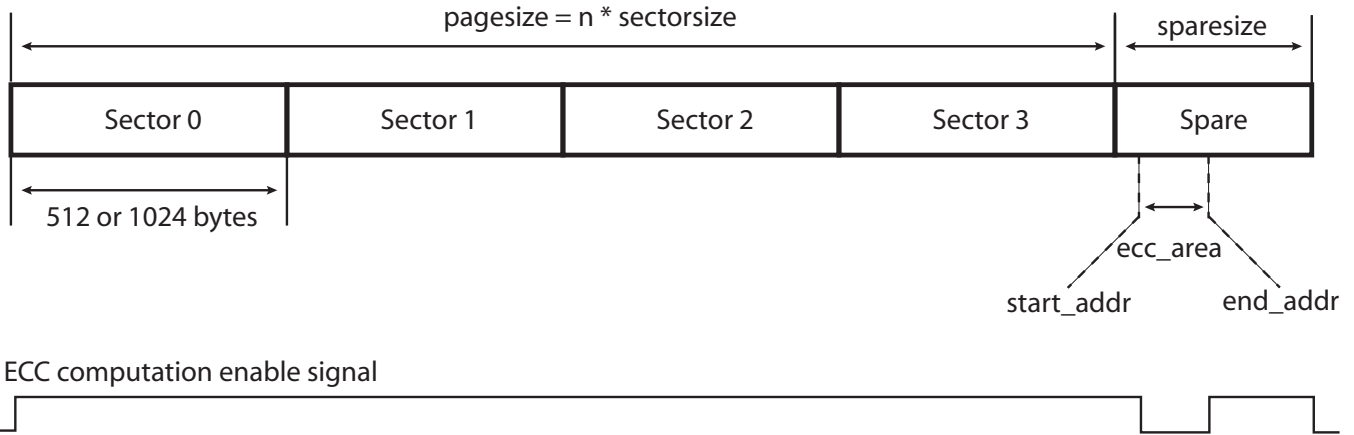
Figure 28-3. NAND Write Operation with Spare Encoding
