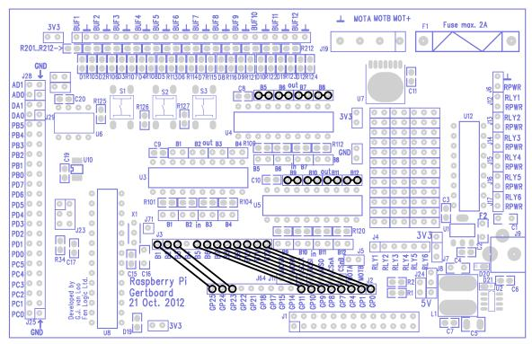
Figure 26: Wiring diagram for the decoder test.
