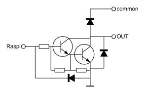
Figure 15: Circuit diagram of each open collector driver.
