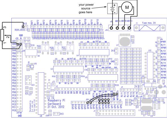
Figure 25: Wiring diagram for the potmot test.
