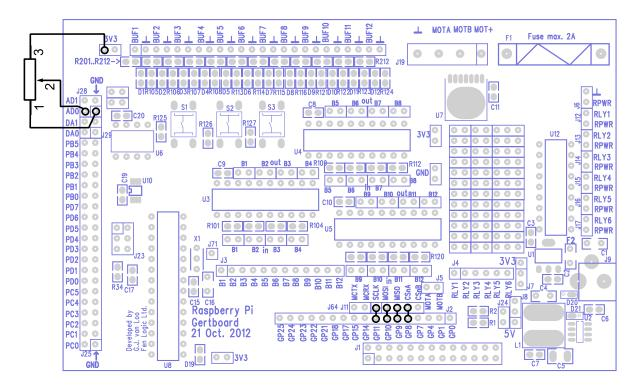
Figure 23: Wiring diagram for the test program atod.
