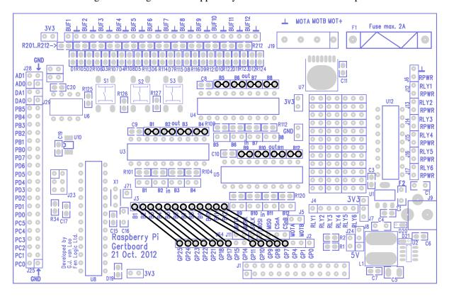
Figure 13: The wiring diagram for the LED test program
