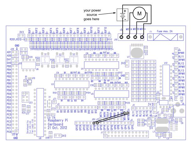
Figure 21: The wiring diagram for the test program motor.
