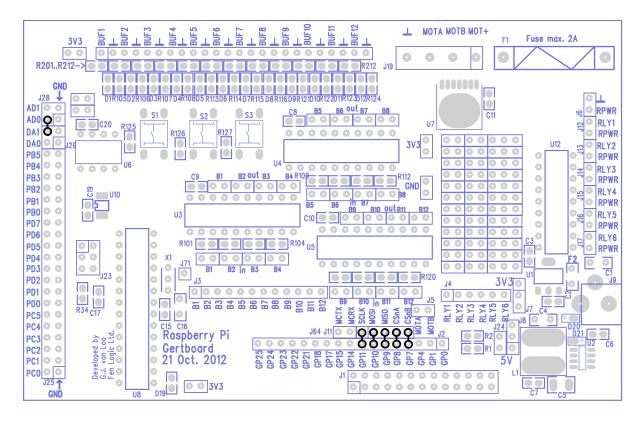
Figure 24: The wiring diagram for the dad test, which allows you to test the A/D and D/A converters together, without the aid of a multimeter or potentiometer.
