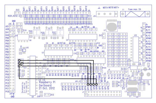
Figure 27: The wiring diagram for uploading sketches to the ATmega microprocessor.
