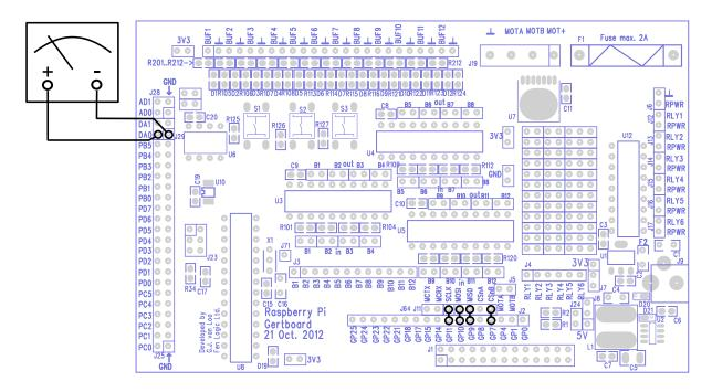
Figure 22: The wiring diagram for the dtoa test.
