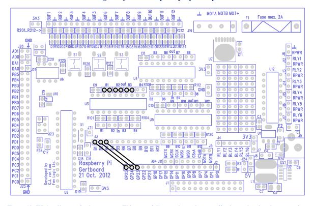
Figure 12: Wiring diagram for buttons test. This type of diagram is much more effective at showing the connections that need to be made, so from now on, we will use these diagrams to show wiring arrangements.
