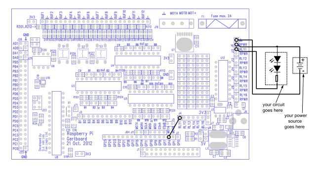
Figure 16: Wiring diagram to test the open collector drivers. On the right is a small test circuit made up of two LEDs in series with a 90  $\Omega$  resistor, and a 9V battery acting as power supply.
