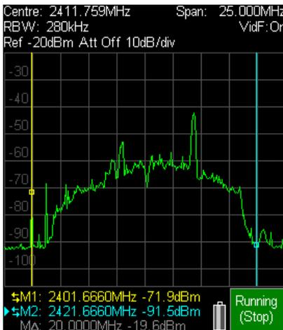
The markers can be set to specified frequency values, scrolled across the screen, or set to automatically find peaks.
