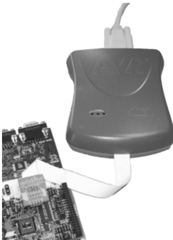
Figure 1-4. Emulating with JTAG ICE
