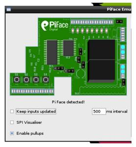
Toggle **Output Pin 1** on by clicking on it. The PiFace interface will click as the relay turns on and the corresponding LED will illuminate. Notice the graphic onscreen updates to show the LED being on, the contacts have changed over on the relay and the first output pin is on.
