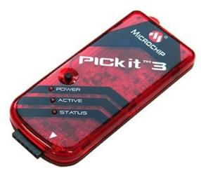
target via an Microchip debug (RJ-11) connector (compatible with MPLAB ICD 2, MPLAB ICD 3 and MPLAB REAL ICE). The connector uses two device I/O pins and the reset line to implement in-circuit debugging and In-Circuit Serial Programming™.
