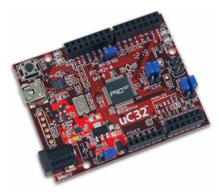
The uC32 can be programmed using the Multi-Platform Integrated Development Environment (MPIDE), an environment based on the original Arduino IDE modified to support PIC32. It contains everything needed to start developing embedded applications. In addition, the uC32 is fully compatible with the advanced Microchip MPLAB® IDE and the PICKit3 in-system programmer/debugger.
