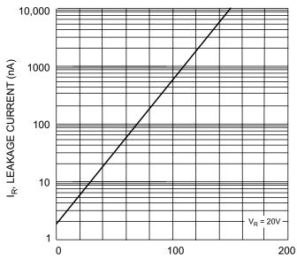
T<sub>j</sub>, JUNCTION TEMPERATURE (°C) Fig. 2 Leakage Current vs Junction Temperature
