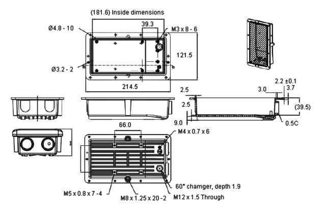
A highly customizable IP67 rated enclosure designed for wireless and industrial control systems in harsh environments. IP67 protection, total protection against dust ingress and the water ingress (water immersion up to 1 meter).
