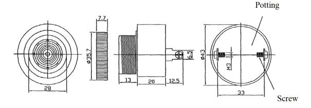
Dimensions: Millimetres Tolerance: ±0.5mm
