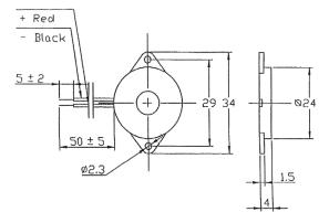
Dimensions: Millimetres Tolerance : ±0.3mm
