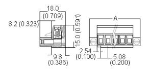
Dimensions: Millimetres (Inches) PCB Layout
