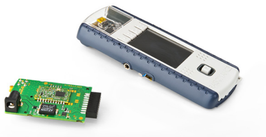
Adeunis RF Bluetooth® extension board & Raisonance Open4 platform
