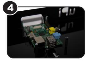
Insert the 2 remaining Pi-Clips, these are located next to Audio and USB sockets on your Pi.
