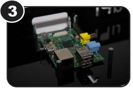
Insert your Raspberry Pi, and slide it into the front Pi-Clips, Note the SD Slot of your Pi should be at the front of the case.
