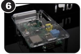
Place the wafer onto the 4 Pi-Clips. Notice the orientation of the wafer on the image above.
