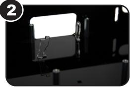
Insert 2 x Pi-Clips into the front of the case, notice the position of the Pi-Clips and also the orientation of the clips.
