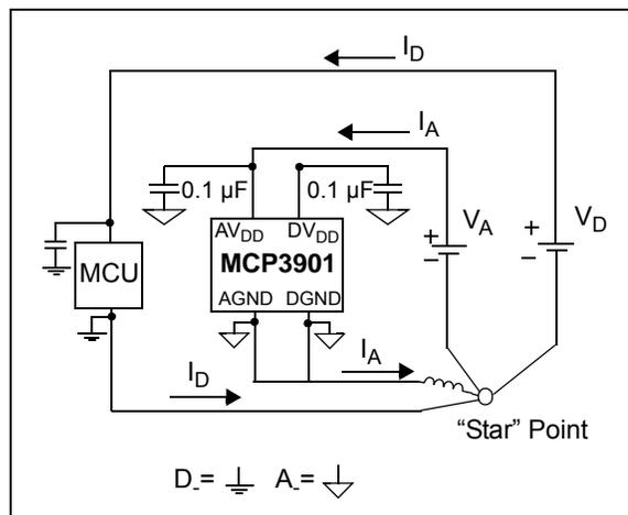
**FIGURE 1:** All Analog And Digital Return Paths Need to Stay Separate with Proper Bypass Capacitors.
