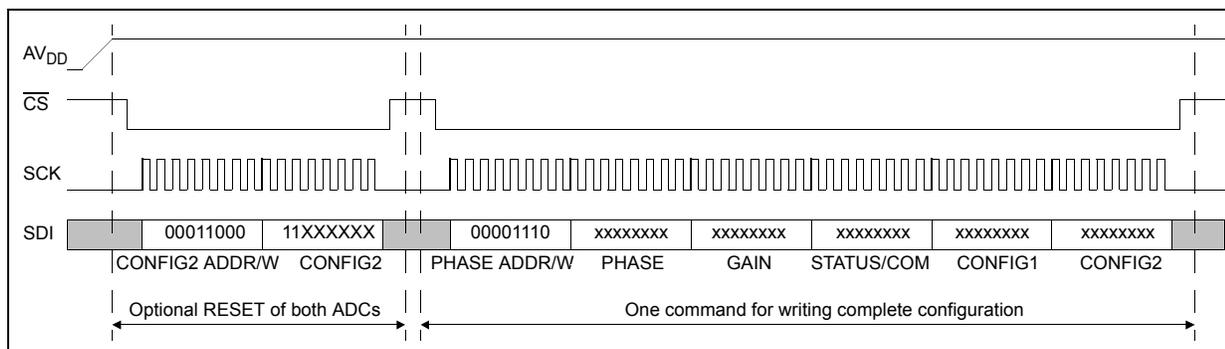
**FIGURE 8:** Configuration Sequence Using Write3901Config(); & Write3901All(); Commands at POR for Fastest Configuration.
