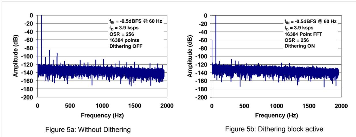
**FIGURE 5:** FFT Analysis Showing Effect of Dithering on Correlated Signals Or Spurs In The Frequency Domain.
