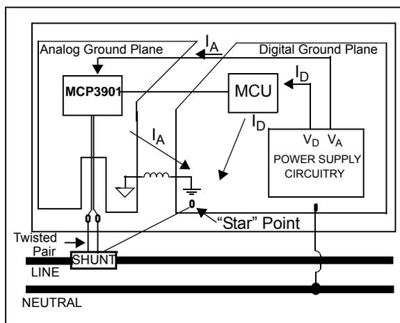
**FIGURE 2:** MCP3901 Design with Proper Analog and Digital Grounding and Power Supply Layout.
