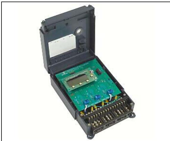
**FIGURE 1:** PIC18F2520 With MCP3909 Meter Showing Line/load Connections To Test Equipment.
