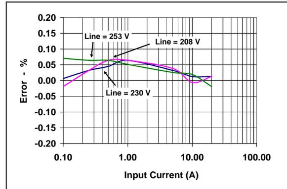
**FIGURE 3:** Meter Accuracy, Voltage Variation Testing.
