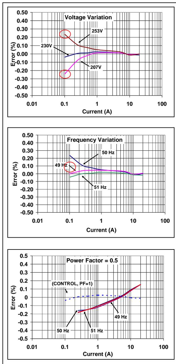
**FIGURE 7:** Hardware and Firmware Improvements Fixed the Areas of Concern (circled in red). This data is from meter revision 1.
