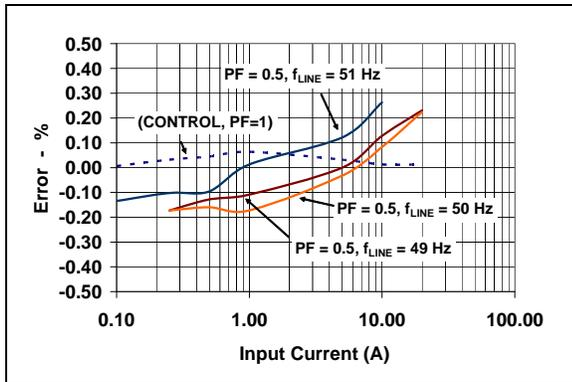
**FIGURE 5:** Meter Accuracy, Frequency Variation Testing.
