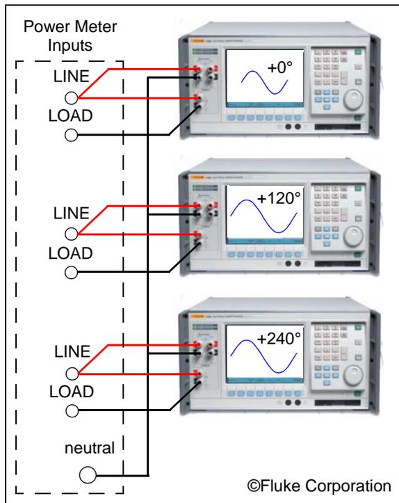
**FIGURE 2:** Meter Calibration Setup.
