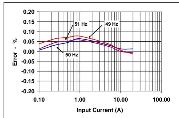
**FIGURE 4:** Meter Accuracy, Frequency Variation Testing.
