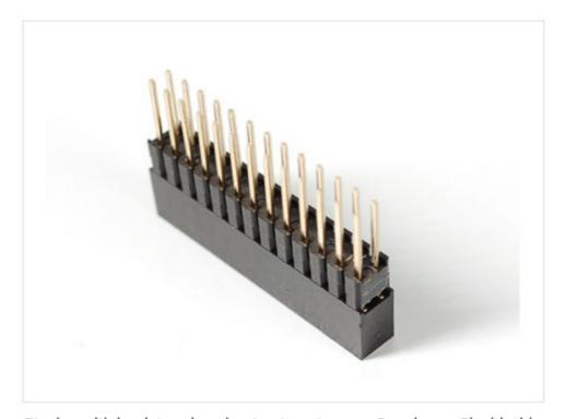
Stack multiple plates, breakouts etc onto your Raspberry Pi with this custom-made extra-tall and extra-long 2x13 female header. The female header part has extra spaces to make it 13.6mm tall: when placed on your Pi, a PCB will clear the Ethernet and USB jacks. The stacky pin part is also extra-long, 9.7mm, so that when a standard 1.5mm thickness PCB is installed, there will be 8mm remaining, plenty to plug into.
