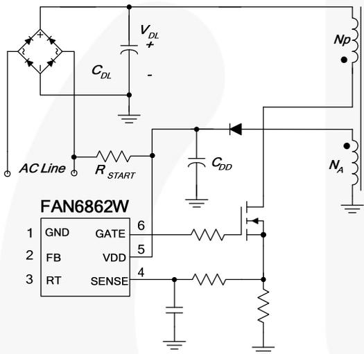
Figure 24. Startup Circuit
