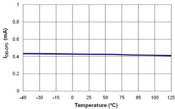
**Figure 8. Operating Current (I<sub>DD-OP2</sub>) vs. Temperature**
