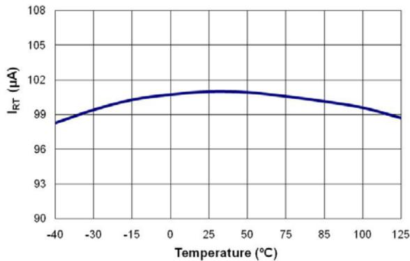
**Figure 22. Output Current of RT Pin (I<sub>RT</sub>) vs. Temperature**
