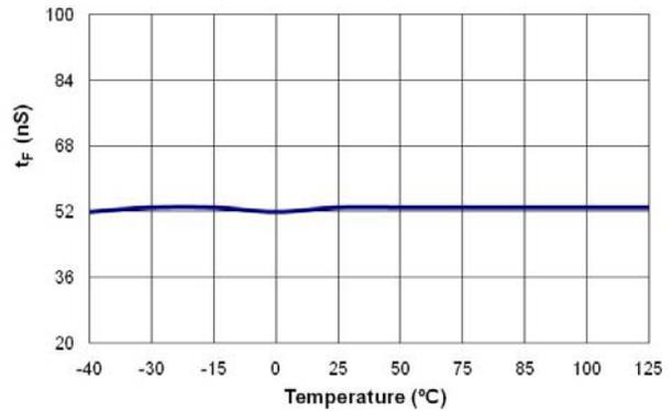
**Figure 21. Falling Time (t<sub>F</sub>) vs. Temperature**
