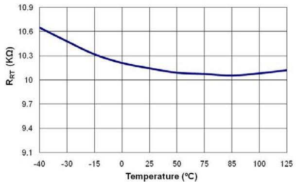
**Figure 23. Maximum External Resistance of RT Pin to Trigger Protection (R<sub>RT</sub>) vs. Temperature**
