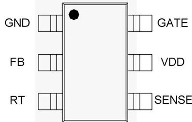
Figure 4. Pin Configuration
