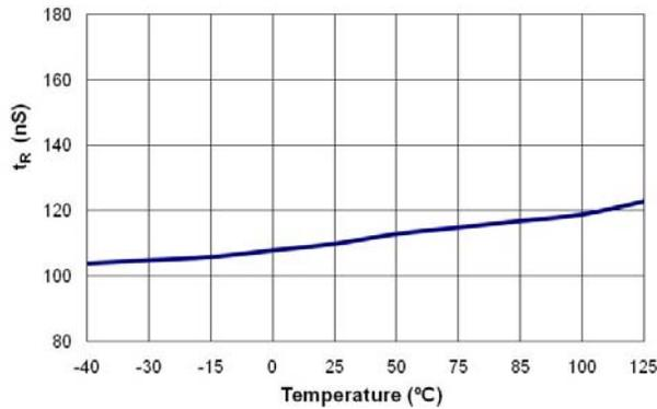
**Figure 20. Rising Time (t<sub>R</sub>) vs. Temperature**
