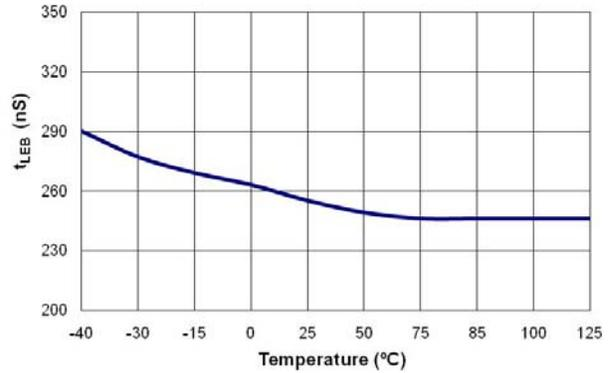
**Figure 19. Leading-Edge Blanking Time (t<sub>LEB</sub>) vs. Temperature**
