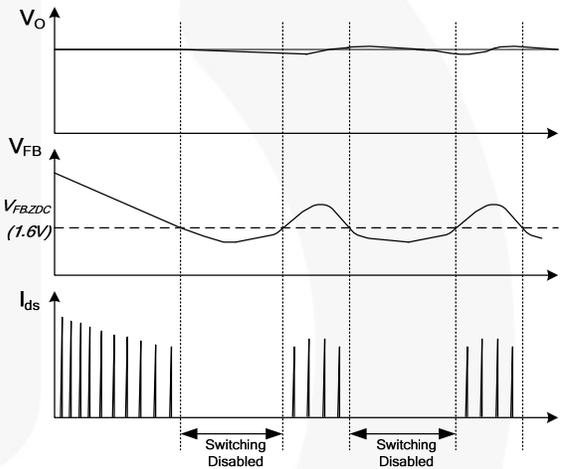
Figure 26. Burst-Mode Operation
