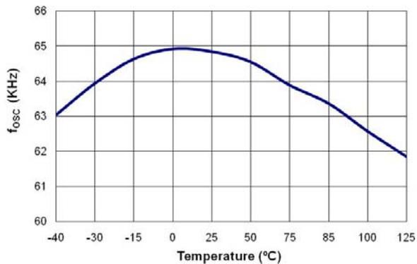
**Figure 10. Center Frequency (f<sub>OSC</sub>) vs. Temperature**
