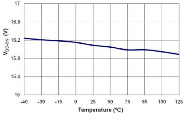
**Figure 6. Turn-On Threshold Voltage (V<sub>DD-ON</sub>) vs. Temperature**
