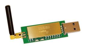
Utilising proprietary LPRS easyRadio technology operating in the 868MHz (UK & Europe) & 915MHz (US) Industrial Scientific & Medical (ISM) bands the Connect2Pi USB 'dongle' provides a simple 'wireless bridge' between Raspberry Pi (Pi2Pi), a Raspberry Pi and a PC or any other device that supports USB serial communications.
