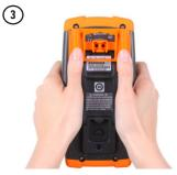
Use both thumbs to fasten the bracket securely to the back of the Agilent U1240 Series Handheld Digital Multimeter.
