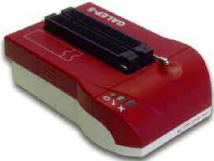
GALEP-5 is a professional palm-sized field programmer with universal I/O capability
