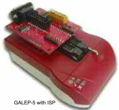
GALEP-5 is a professional palm-sized field programmer with universal I/O capability
