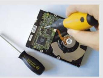
...in electronic assemblies and ESD protected zones, where electrostatic sensitive components and devices must be grounded, the TorqueVario®-S ESD should be used.
