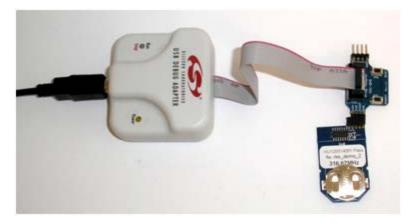
In this setup, the user can incorporate the debugging capabilities into the final application using a cheap 4-pin header connection.
