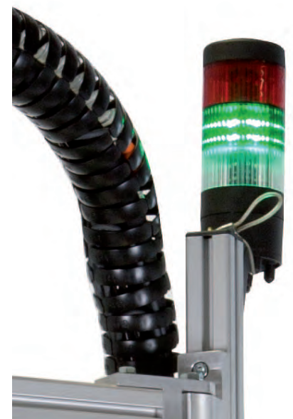
Signal lamps indicate the operating status
