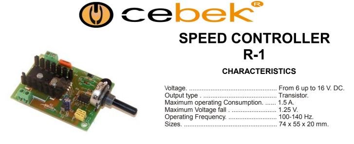
The R-1 module is a speed controller for DC motors, supplied from 6 up to 16 V. DC with a maximum consumption of 1.5 A. The speed adjustment is done thanks to the variation of the duty cycle. The module could also control other resistive loads like resistors.
