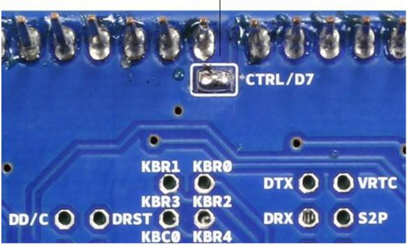
Several of the modem pins are exposed on the underside of the board. These provide access to the modem for features like speaker output and microphone input. See the datasheet for complete information.
